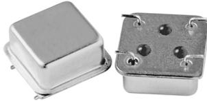
The XOSM-52 series oscillator is half size, has tri-state enable/disable controlled function. The metal package with pin 4 case ground acts as shielding to minimize EMI radiation.
