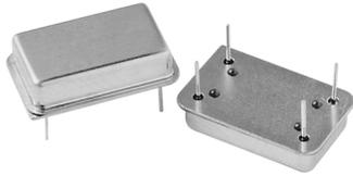
The XO-53 series oscillator is TTL compatible and features fast rise/fall times with high reliability at low cost. The metal package with pin 7 case ground acts as shielding to minimize EMI radiation.
