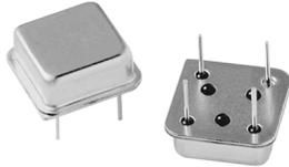
The XO-52 series oscillator is half size, has tri-state enable/disable controlled function. The metal package with pin 4 case ground acts as shielding to minimize EMI radiation.
