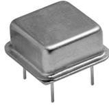
The XO-523 series oscillator is half size, has tri-state enable/disable controlled function, and is with a 3.3 V power supply voltage. The metal package with pin 4 case ground acts as shielding to minimize EMI radiation.
